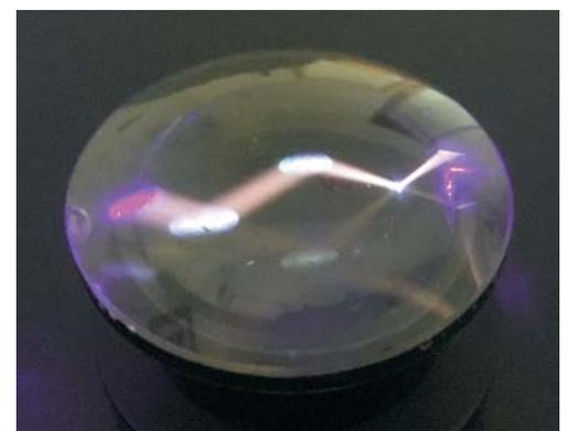
Fig.3. Origination of stray light in optical lens. Light of 405 nm laser pointer is invisible in clean air, but visualized at the surface and in the bulk of the lens due to scatter, reflections, and auto-fluorescence.
