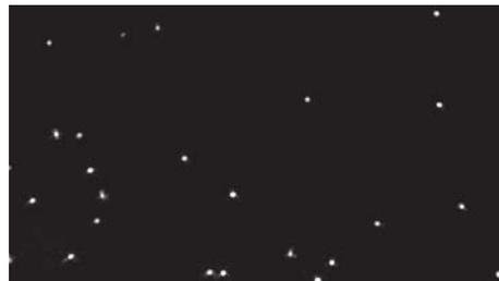
Fig.8. Lightguide-based TIRF,100X, NA 1.0 water-imm.objective. 1-um fluorescent beads.
